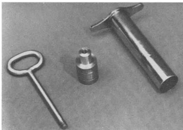
FIG. 5. Disassembled sampler for use with plastic fat sample holder.
